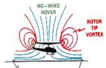
creates a high velocity flow pattern flowing down through the rotor disk and out in all directions. A rotor vortex also develops around the entire tip path of the rotor disk. These flow patterns can persist, in place, after the helicopter departs and they are capable of upsetting light aircraft in the vicinity.
